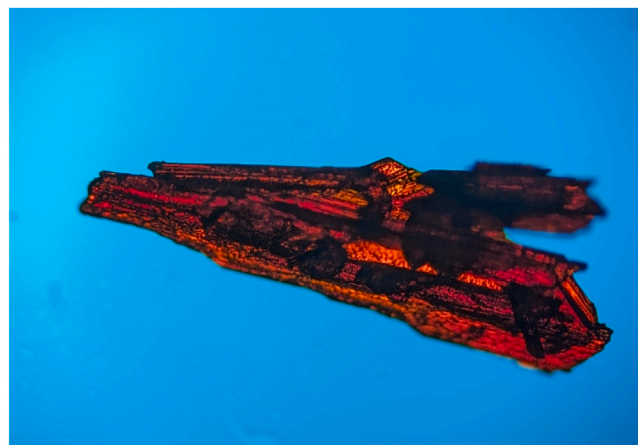
Fig. 1. Picture of [(\text{C}_3\text{H}_7)_4\text{N}]\text{FeBr}_4 crystals, taken under polarized light with 50\times amplification.
