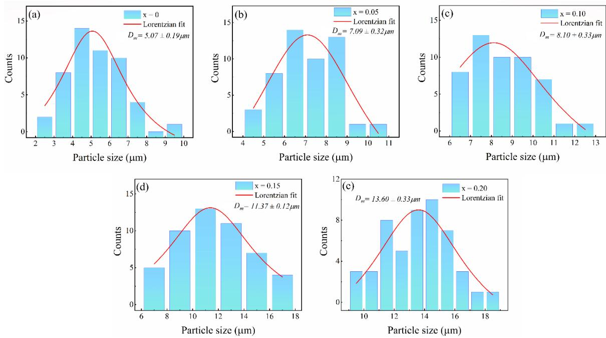
Fig. S4: Size distribution histograms obtained from SEM images for  $\text{Fe}_{(1-x)}\text{Co}_x\text{NbO}_4$  samples ( $0.05 \leq x \leq 0.20$ ). (a)  $x = 0$ , (b)  $x = 0.05$ , (c)  $x = 0.10$ , (d)  $x = 0.15$  and (e)  $x = 0.20$ .
