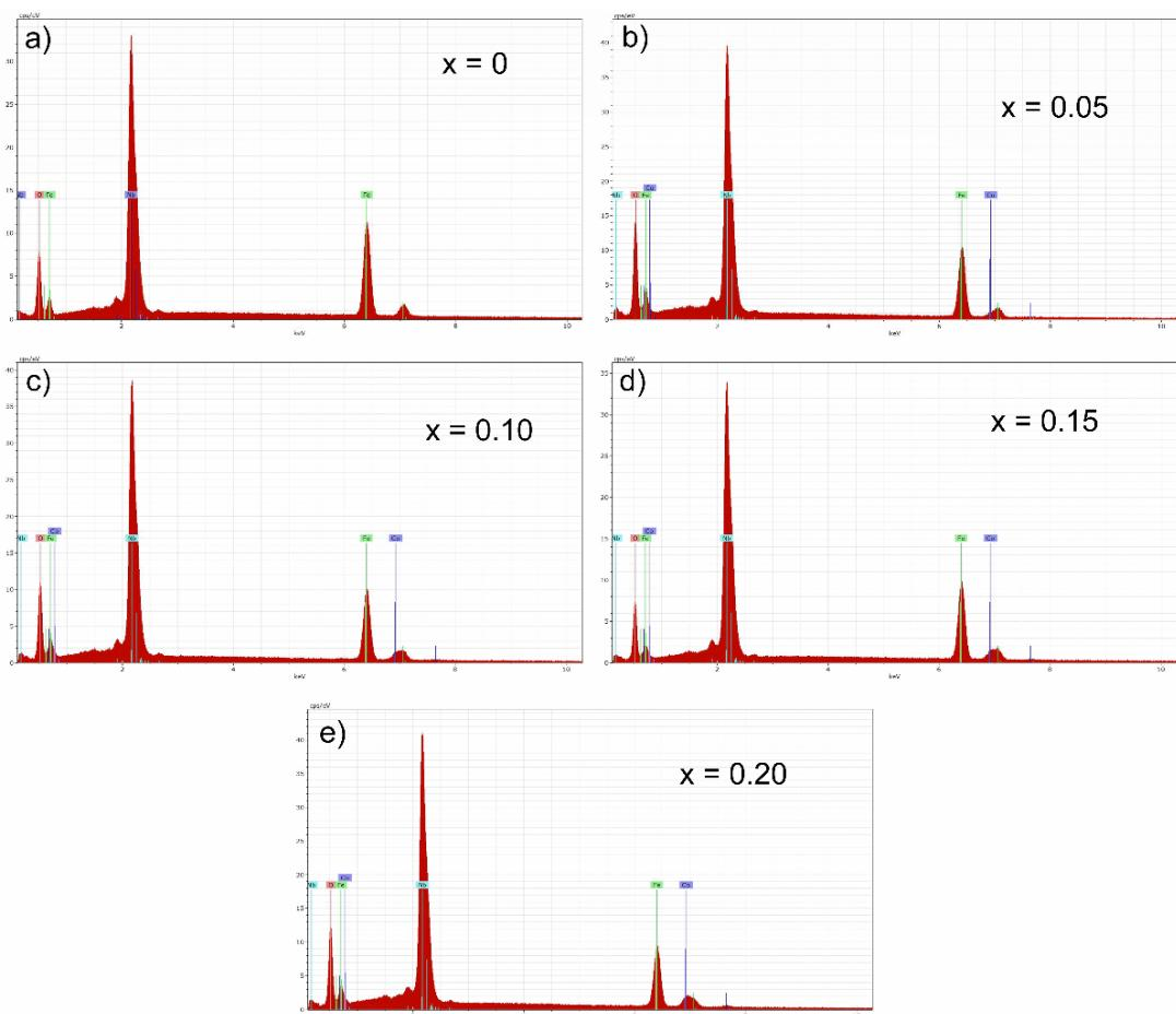
Fig. S5: EDS spectra for  $\text{Fe}_{(1-x)}\text{Co}_x\text{NbO}_4$  polycrystalline. (a)  $x = 0.0$ , (b)  $x = 0.05$ , (c)  $x = 0.10$ , (d)  $x = 0.15$  and (e)  $x = 0.20$ .
