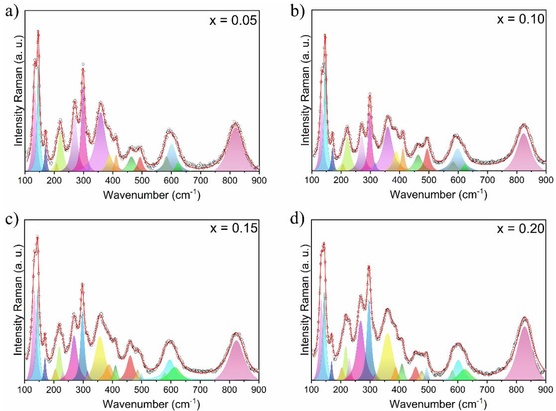
Fig. S3: Deconvolution profile of the Raman modes for  $Fe_{(1-x)}Co_xNbO_4$  samples ( $0.05 \leq x \leq 0.20$ ). (a)  $x = 0.05$ , (b)  $x = 0.10$ , (c)  $x = 0.15$ , (d)  $x = 0.20$ .
